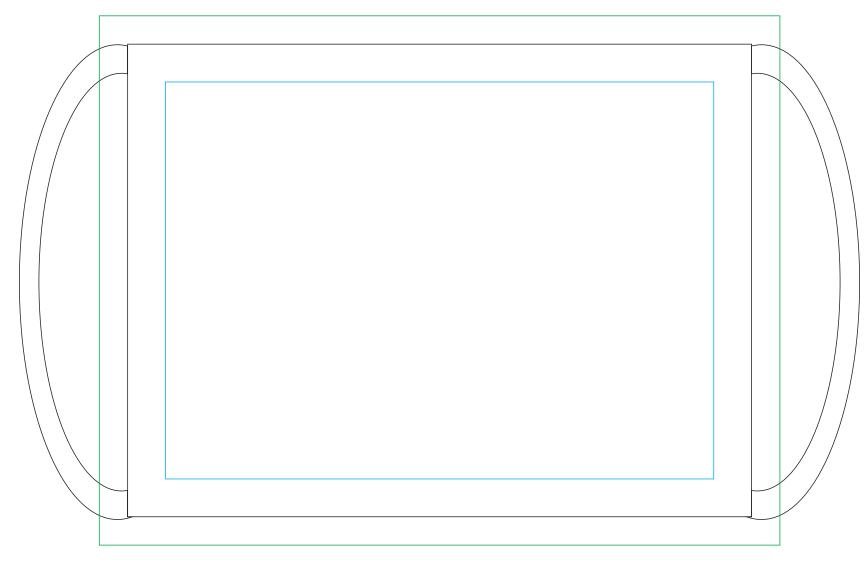
Green Line is for bleed, please fill up to this line to allow for movement Blue line is the safety zone, this area 100% safe from being cut off
